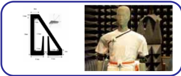
Development of a small antenna for BAN and propagation measurement using body-fantom
